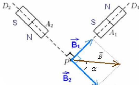
$$B = \sqrt{B_1^2 + B_2^2} = \sqrt{30^2 + 40^2} = 50\text{mT} = 0,5\text{T} \quad (2)$$
