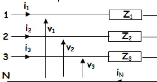
$$\underline{I}_N = \underline{I}_1 + \underline{I}_2 + \underline{I}_3 = \frac{V_1}{Z_1} + \frac{V_2}{Z_2} + \frac{V_3}{Z_3}$$
